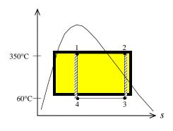
(c) The net work can be determined by calculating the enclosed area on the T-s diagram,
