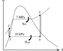
**8-121** A steam power plant that operates on an ideal reheat Rankine cycle between the specified pressure limits is considered. The pressure at which reheating takes place, the total rate of heat input in the boiler, and the thermal efficiency of the cycle are to be determined.
